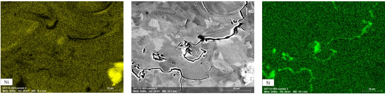
Figure 5 – EDS elemental maps for sample 3 ( P=150W , v_s=800mm ), showing undissolved Ni and Si segregations associated with hot cracks.
