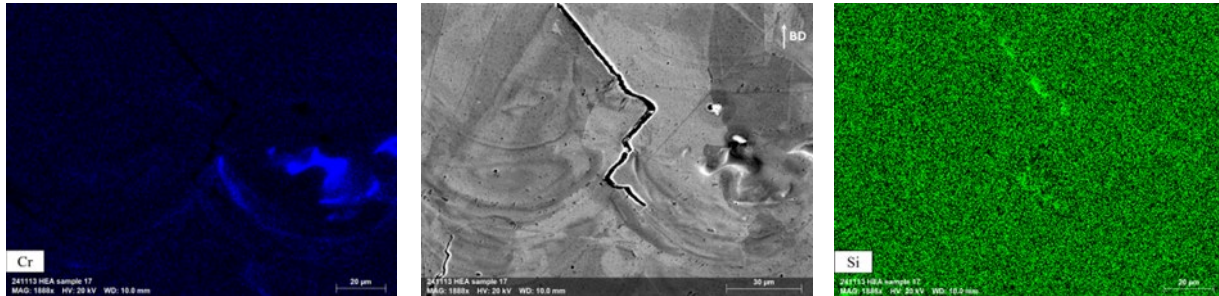
Figure 6 – EDS elemental maps for sample 17 ( P=175W , v_s=800mm/s , remelting), showing undissolved Cr and Si segregations associated with hot cracks.
