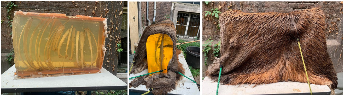
Fig. 5 A realistic target made of a sequence of horse ribs that are encased in ballistic gel and covered with fresh deer hide. The wooden frame (left) was removed before the experiment and the hide was maintained under tension by turnbuckles attached at the sides and the back
