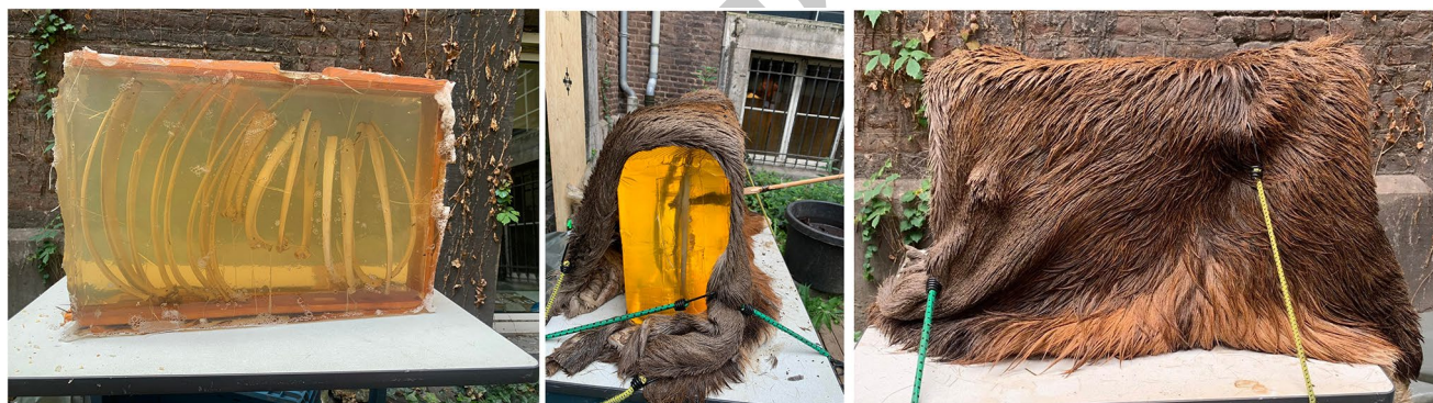
Fig. 5 A realistic target made of a sequence of horse ribs that are encased in ballistic gel and covered with fresh deer hide. The wooden frame (left) was removed before the experiment and the hide was maintained under tension by turnbuckles attached at the sides and the back
