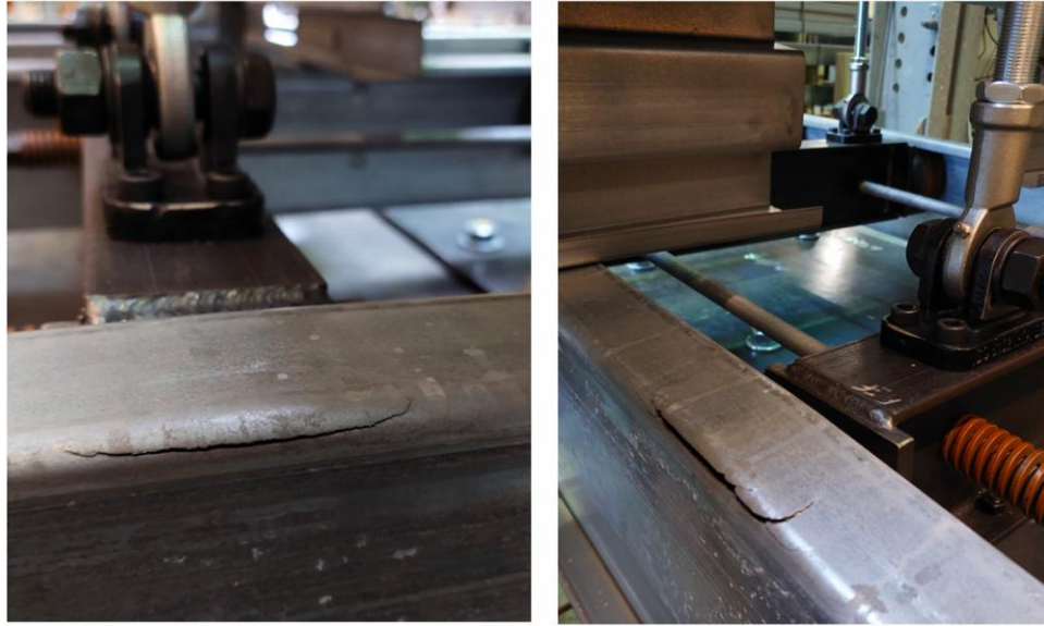
Fig. 17. Fatigue crack for (a) specimen S2 and (b) specimen S4.
