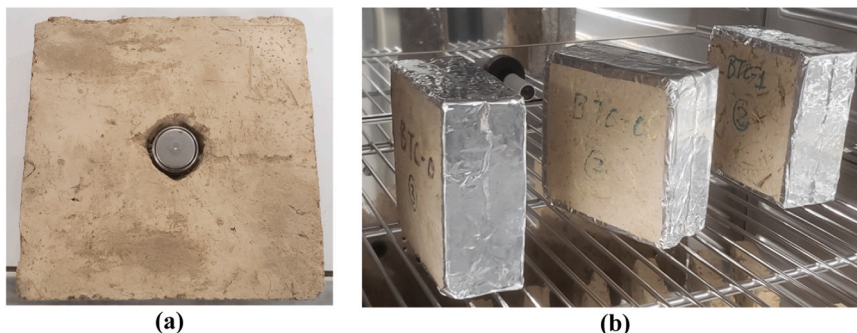
Fig. 4. (a) Sample with hygro-button; (b) Sample + hygro-button assembly.
