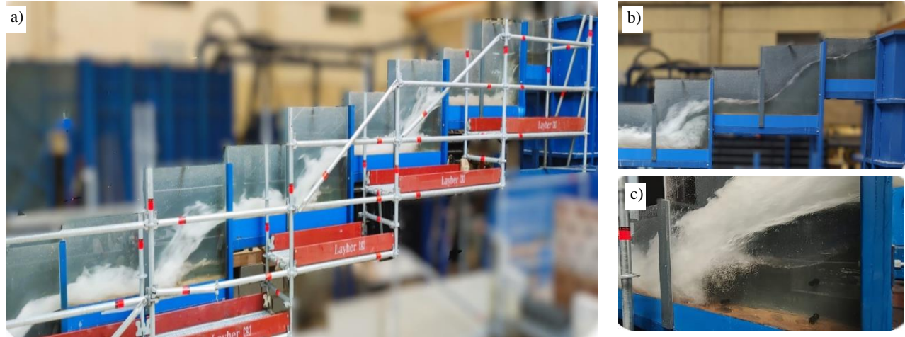
Figure 3. Flow conditions a) over the whole model at flow rate of 0.2 \text{ m}^2/\text{s} , b) at steps I and II at flow rate of 0.6 \text{ m}^2/\text{s} , and c) in the cavity of step IV at flow rate of 0.4 \text{ m}^2/\text{s} .
