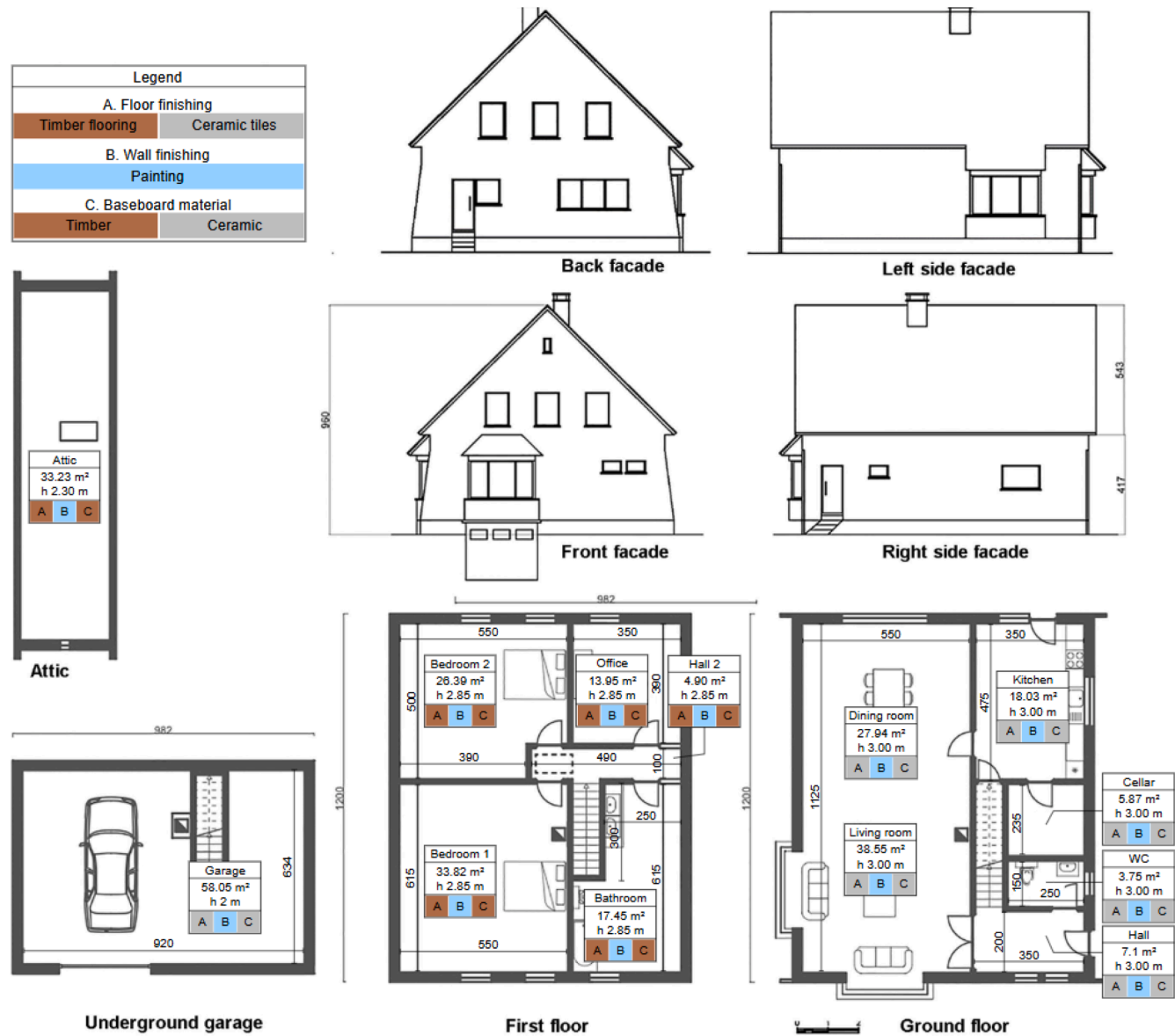
Fig. A.1. Plans and elevations of the single-family house archetype (from Attia et al., [12]).
