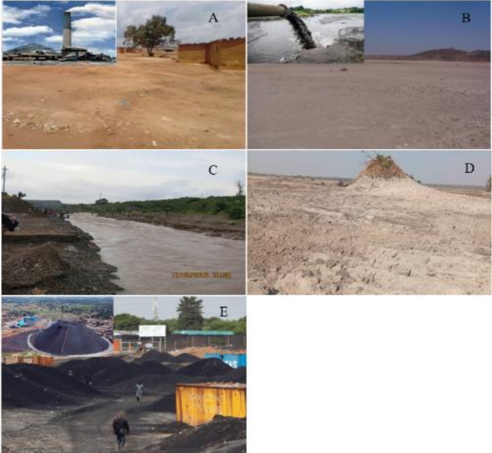
Figure 3-2. Main types of mine tailings, and contaminated soils and sediments in the KCB. (A) Soil contaminated by emissions from the smelter, (B) wastes from concentrates of Cu and Zn sulfides by Environments 2024, 11, 122 4 of 18 flotation, (C) river sediments contaminated by wastes released by mining plants, (D) wastes from concentrates of Cu and Co oxides, (E) slag from the smelting process of copper.
