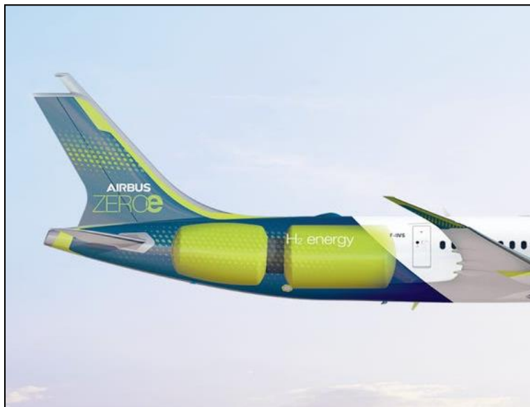
Airbus ZEROe hydrogen tanks design.
