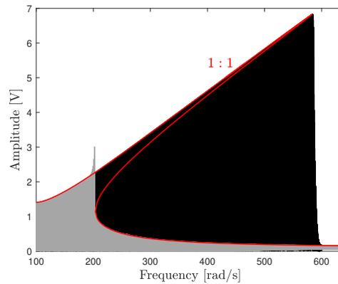
Figure 6: FRC around the 2 : 1, 3 : 1, and 1 : 1 resonances of the electronic Duffing oscillator at  $p = 2$  [V]. The (x-)ACBC results (—) are compared with swept-up (—) and swept-down (—) sine tests.
