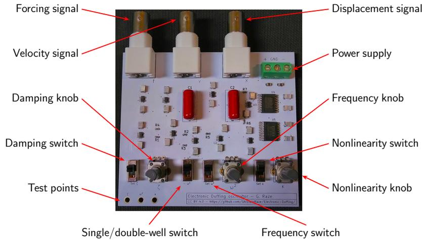
Figure 4: Setup of the electronic Duffing system [7].
