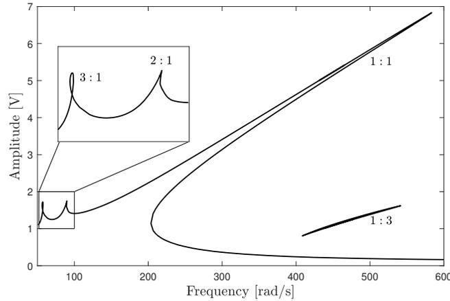
Figure 5: Bifurcation diagram of the Duffing oscillator with a forcing amplitude of 2 [V]. The FRC was identified using ACBC and x-ACBC. Stable and unstable open-loop solutions are represented in the same way.
