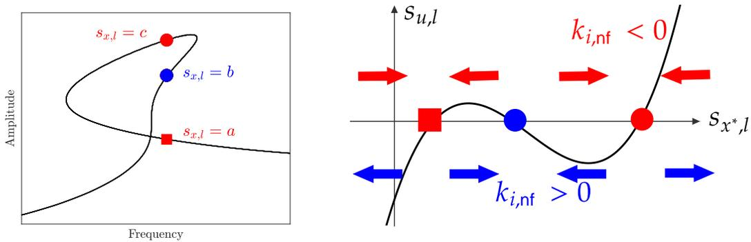
Figure 3: Left: FRC around a secondary resonance, with colored points indicating solutions on different branches of this resonance. Right: Variation of a non-fundamental resonant harmonic Fourier coefficient of the control action,  $s_{u,l}$ , with respect to the controlled non-fundamental resonant harmonic Fourier coefficient of the reference displacement,  $s_{x^*,l}$ .
