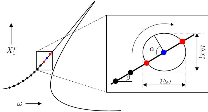
Figure 2: Illustration of the arclength continuation method introduced in [5]. Circles indicate previous responses, the square marks the next response, the blue point is the ellipse’s center, and the red markers are intersections along the arc.
