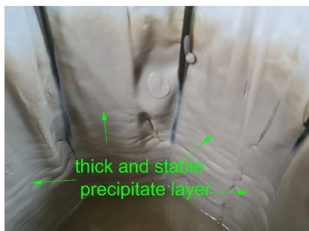
Fig. A 9-2: The thick and stable precipitate layer in the 10 \mu\text{m} pore-size filter plate
