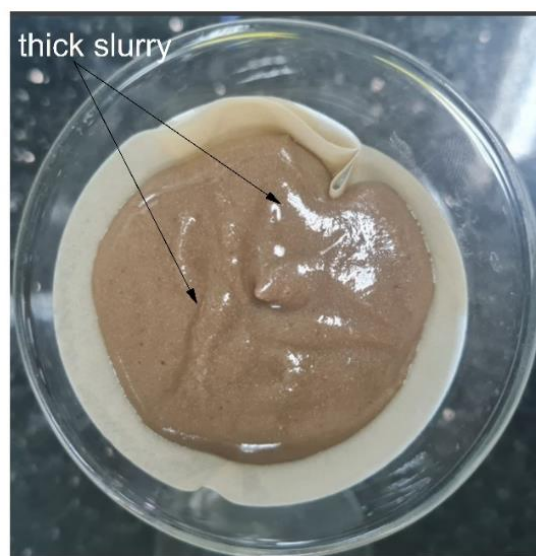
Fig. 6-18: The liquid-solid mixture as thick slurry after leaching at phase ratio 5 mL g -1 , 2M H 2 SO 4 for CHES
