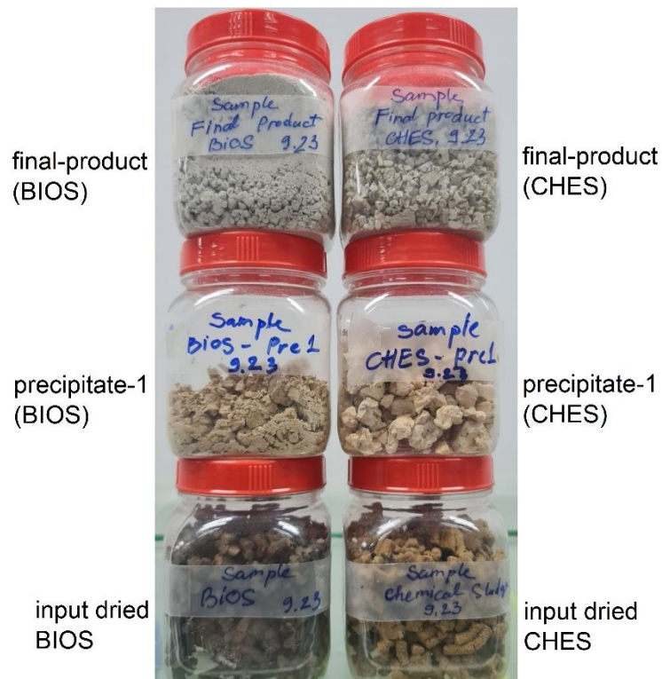
Fig. A 9-6: Images of input dried sludges and products from the P-recovery process
