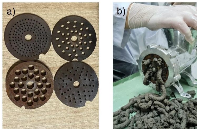
Fig. 6-2: Different pore sizes of extrusion plates (a) and extruder (b)
