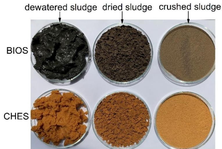
Fig. 6-1: Sludge preparation for digestion
