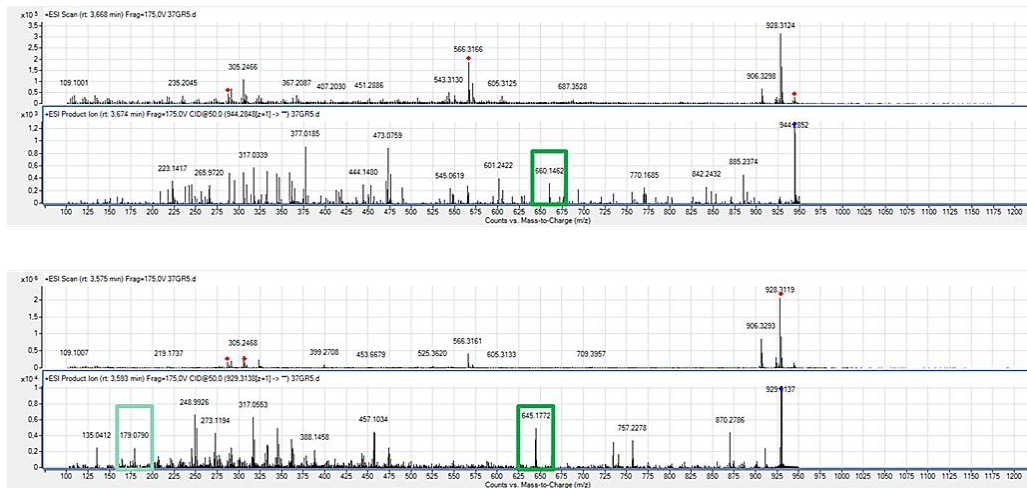
Figure 47: MS/MS spectra of masses at m/z 928.3119 (bottom spectrum, with a fragmentation of m/z 929.3138) and m/z 944.2848 (top spectrum).
