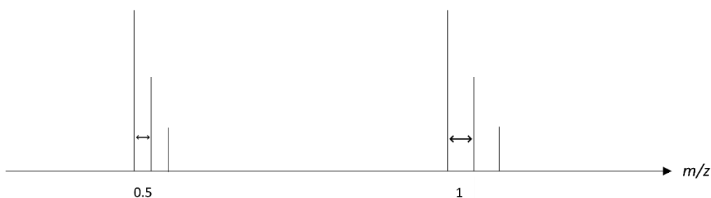
Figure 26: Characteristics of MS spectra of multi-charged compounds.
