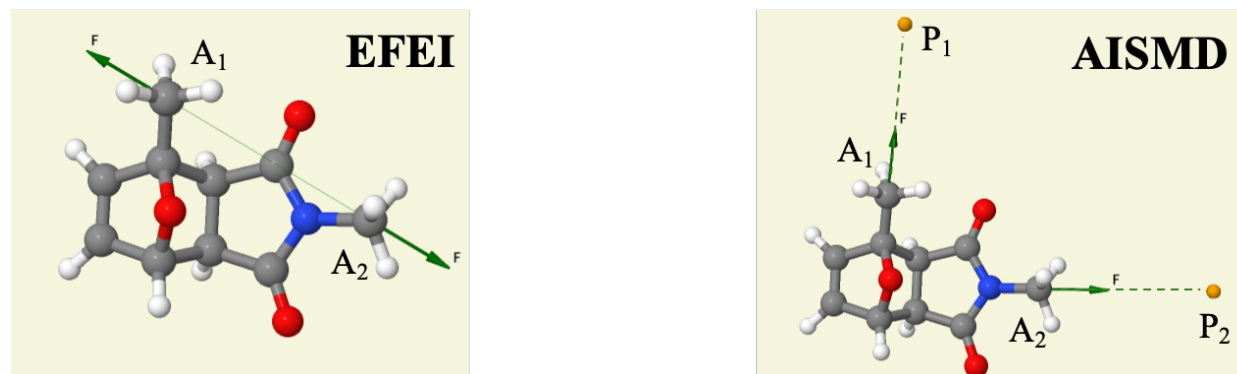
Figure 3.2: Key differences between EFEI and AISMD approaches. In EFEI, the external force is applied along the line that connects the terminal anchoring atoms ( A_1 and A_2 ). In contrast, in AISMD, the force pulls each anchoring atom towards an associated pulling point ( P_1 and P_2 ) in the lab frame.
