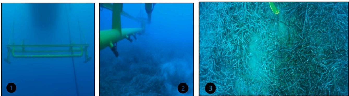
Fig. 6. Cleaning machine (1), water jets (2), efficiency (3). Left part and right part: before and after cleaning operation, respectively.
