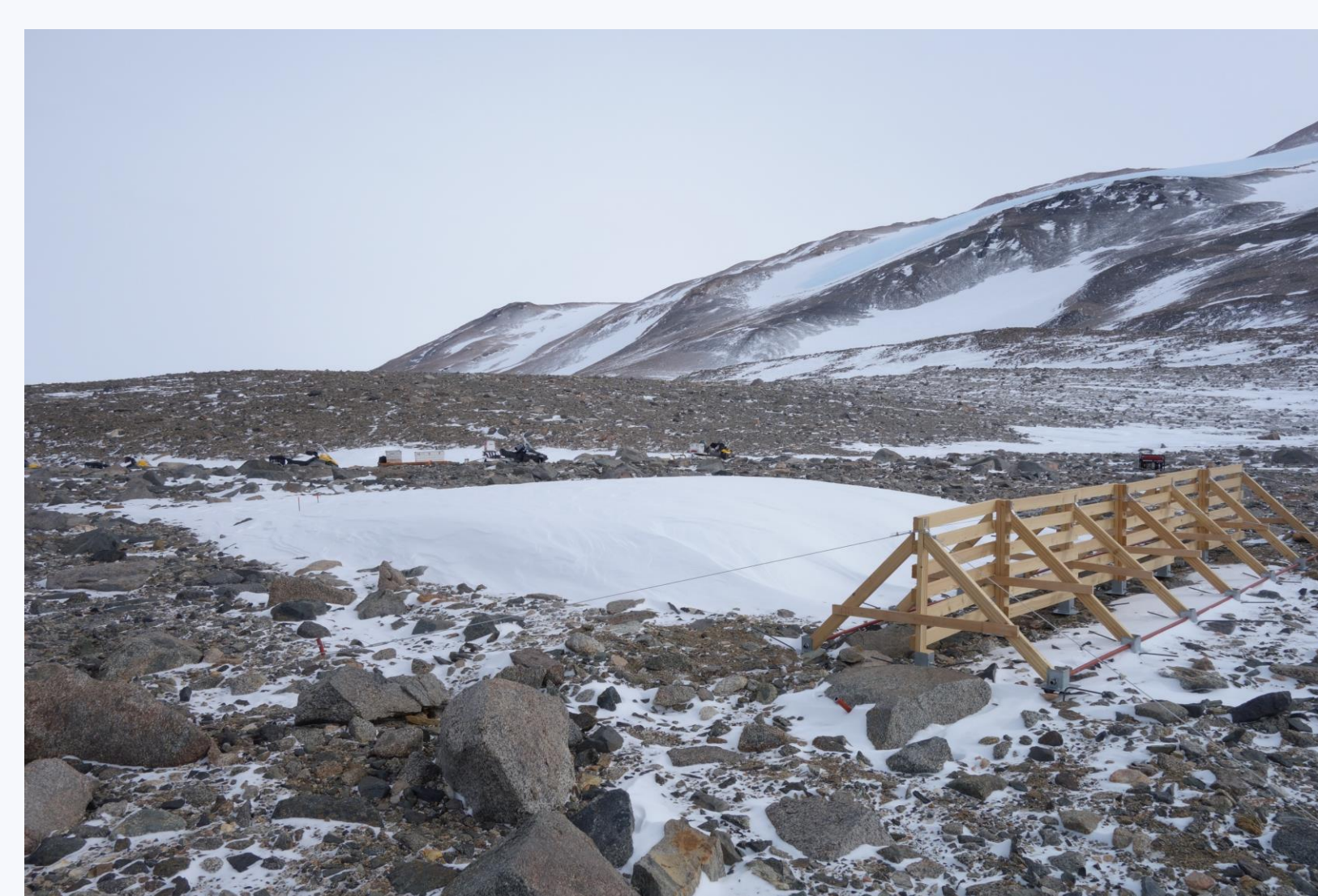
Fig. 5: Snowfence in the Sør Rondane Mountains (East Antarctica). Identical set-ups are installed in Svalbard. Increased snow accumulation will reduce growing season and promote heterotrophic activity, and increased water availability and protection from cold winds.
