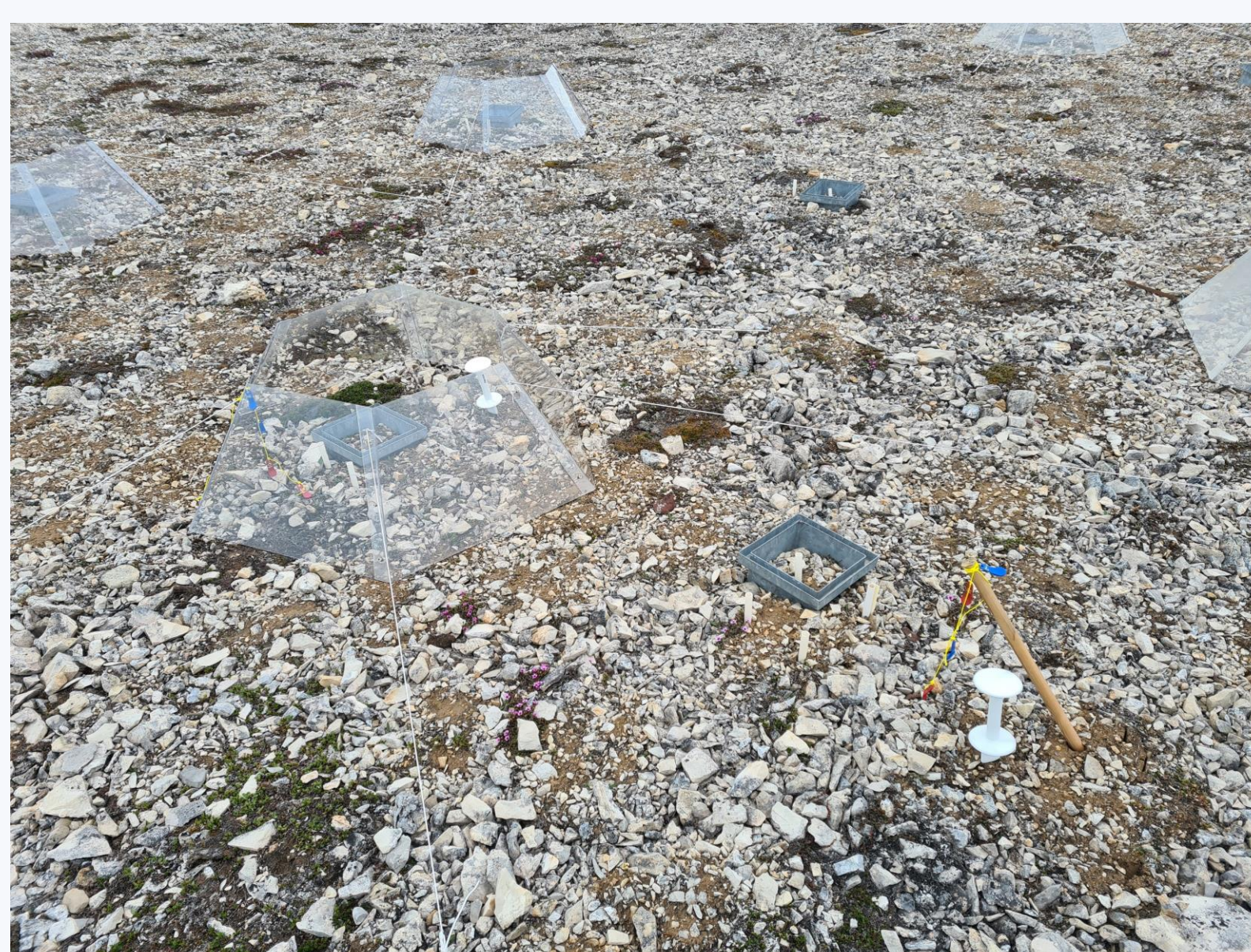
Fig. 4: Open Top Chambers (OTCs) in Svalbard, installed in 2014 by Dr. K. Newsham (BAS). Soil and air temperature is increased inside an OTC. Amplicon and metatranscriptomics HTS will be used to track responses to warming in the taxonomic composition and functioning of tundra microbial communities, incl. bacteria, protists and fungi.
