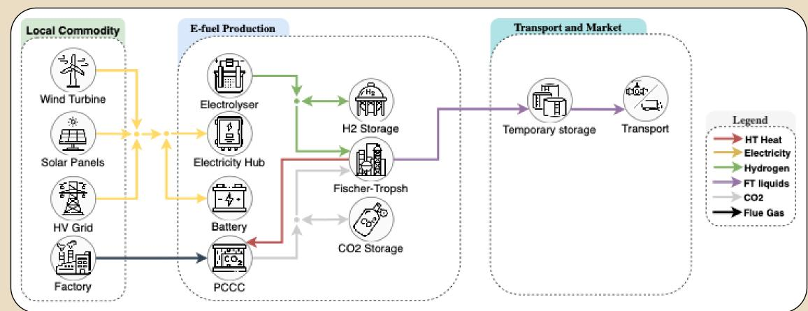
We are considering an industrial site located next to a lime plant that emits a constant flow of CO<sub>2</sub>-rich flue gases equivalent to a capture rate of 9 tCO<sub>2</sub>/hour.
