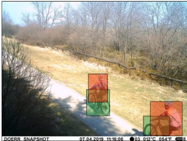
Fig. 2: Example of a processed image from "Botrange" (Bot, HF-E) with bounding boxes for each detected/identified object, in this case two persons (red) and their bikes (green). (For interpretation of the references to color in this figure legend, the reader is referred to the Web version of this article.)
