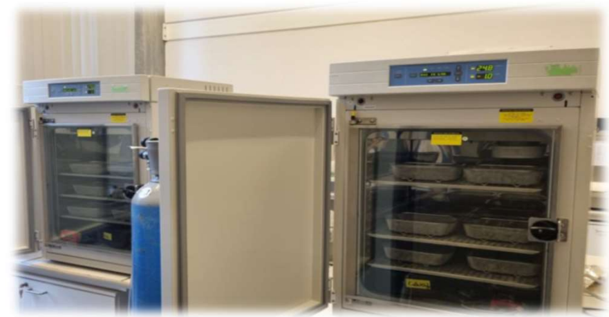
Static carbonation chambers
