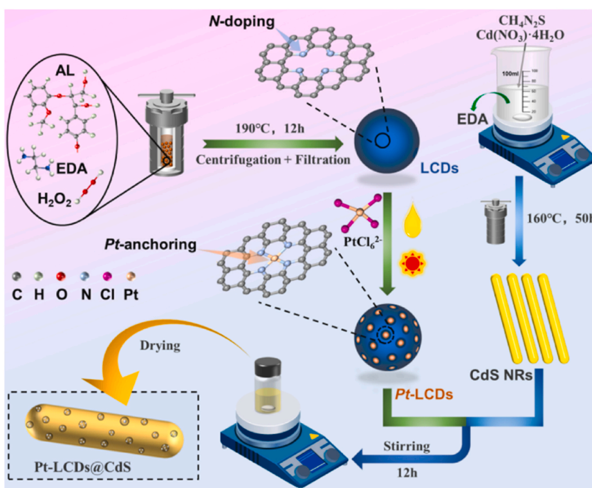
Fig. 11. Overall process for the fabrication of Pt-NLCDs@CdS reported by Zhuang et al. Reprinted with permission from Ref. [60].
