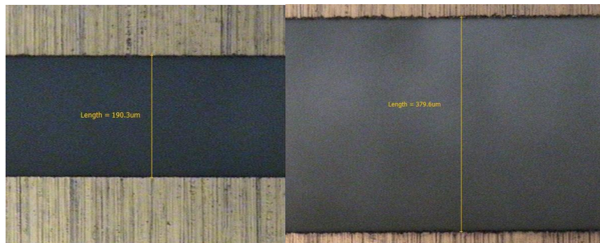
Figure 16. The microscope picture of the 189 \mu\text{m} (left) and 379 \mu\text{m} (right) slits.
