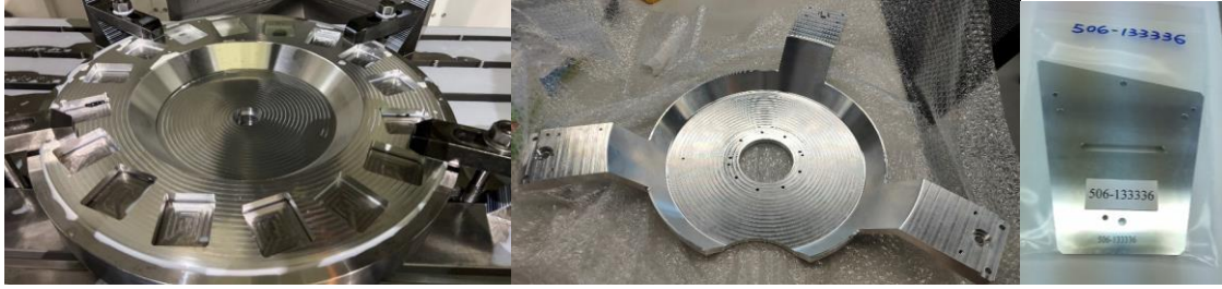
Figure 15. Picture of the FP2 wheel components. The left is the wheel body. The middle panel shows the spider vane and the right panel is a cartridge bed of a slit mask.
