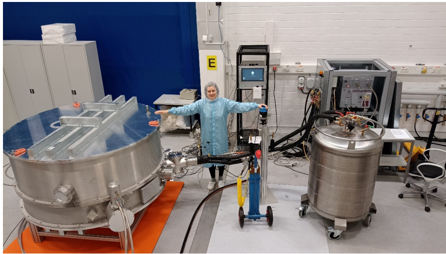
Figure 6. The SCAO test cryostat. It provides the operating environment for the SCAO Module prior to the integration into the METIS cryostat. The cryostat is fully operational and will be used in the subsystem test phase. It forms a test setup in conjunction with the telescope simulator (top left).
