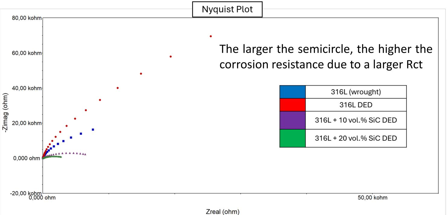
The Nyquist plot is in the shape of a semicircle, and the diameter of the plot gives the charge transfer resistance of the samples.
