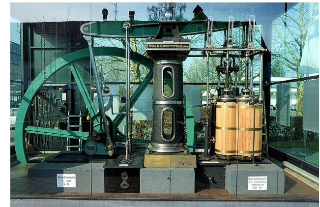
Woolf steam engine 1858 (licensed under the Creative Commons Attribution-Share Alike 2.5 Generic license)
