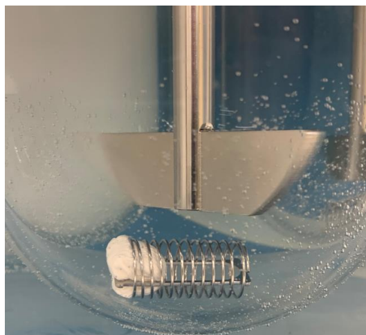
Figure 4 - Gel mass formed by F7 once in contact with the acidic dissolution medium.
