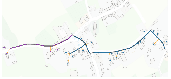
Fig. 2: Considered network which consist of a subpart of the reconstructed Belgian network that have one single substation connected to two-feeders.
