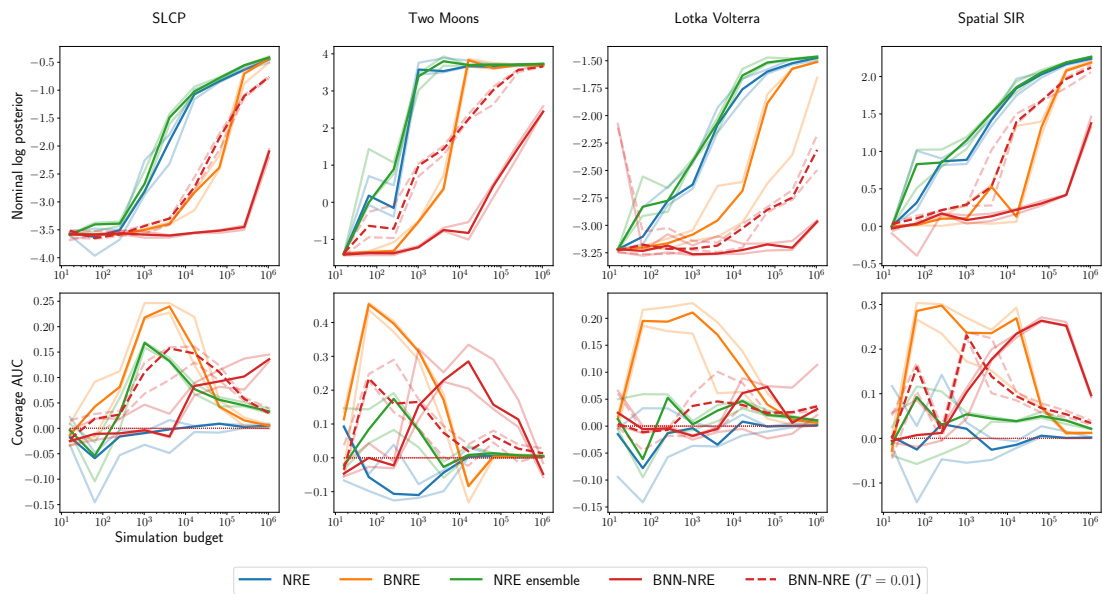
Figure 7.12: Comparison of different NRE simulation-based inference methods through the nominal log probability and coverage area under the curve. The higher the nominal log probability, the more performant the method is. A calibrated posterior approximation exhibits a coverage AUC of 0. A positive coverage AUC indicates conservativeness, and a negative coverage AUC indicates overconfidence. 3 runs are performed. The median run is reported in plain, and the shaded lines represent the other two runs.
