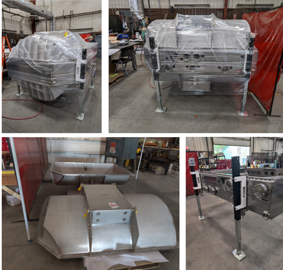
Figure 3. SCALES cryostat at Cameron MD. Top: The cryostat in protective plastic wrap. Bottom left: The top (foreground) and bottom (background) lids. Bottom right: The load ring on its jack stands. Photo credit: B. Blank (PulseRay), RDS.
