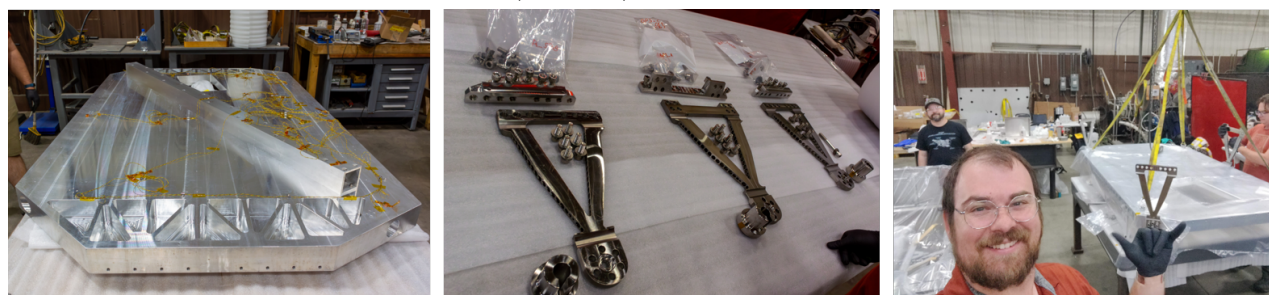
Figure 5. The SCALES bench. Left: The underside of SCALES with its temperature sensors. Middle: The three titanium bipods and pins that support the bench. Right: Test-fitting the bench to the load ring. Photo credits: M. Gonzales, RDS.
