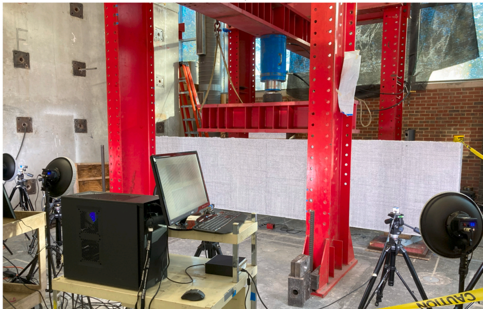
Fig. 2. a) Geometric and reinforcement details for CCR1-CCR6 (Note: All dimensions are in mm). b) Collecting deformation data using full field-of-view DIC on the west face of the specimens.
