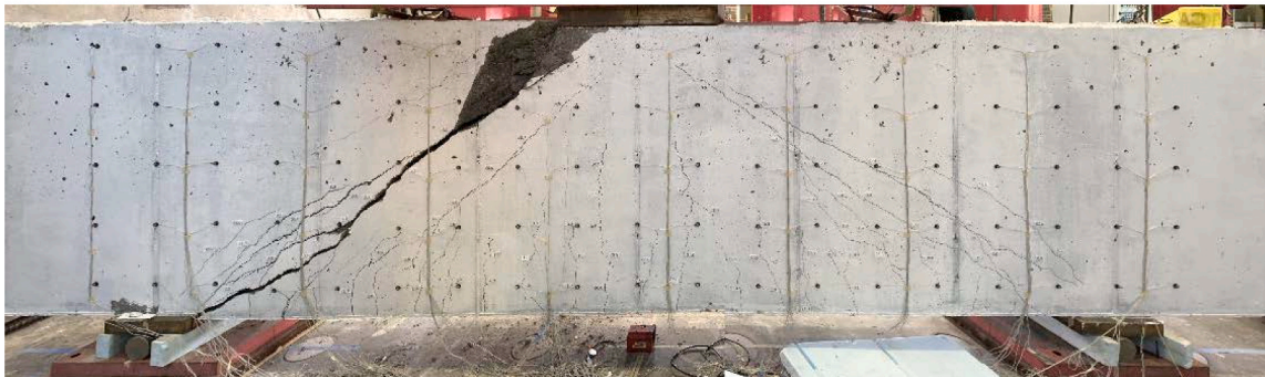
c) Specimen CCR2 after failure
