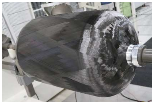
Figure 1. COPV produced by filament winding.
