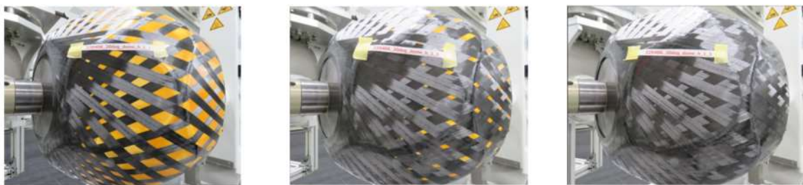
Figure 2. Specific mandrel with flat faces: detail of the filament winding process and tape interlacement at the dome area
