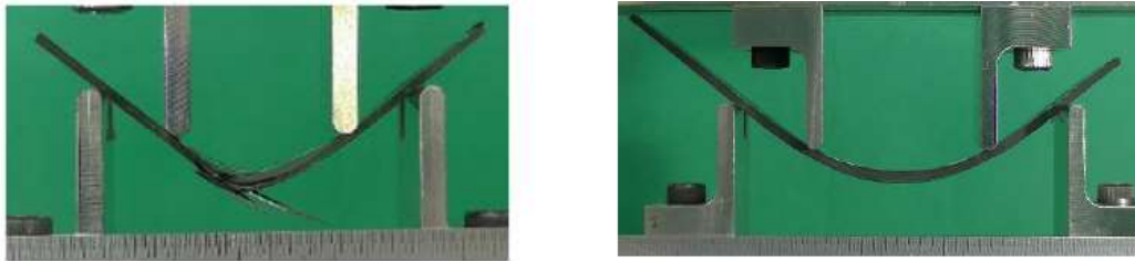
Figure 6. Physical testing on coupons extracted from the dome area (left: longitudinal direction; right: circumferential direction)
