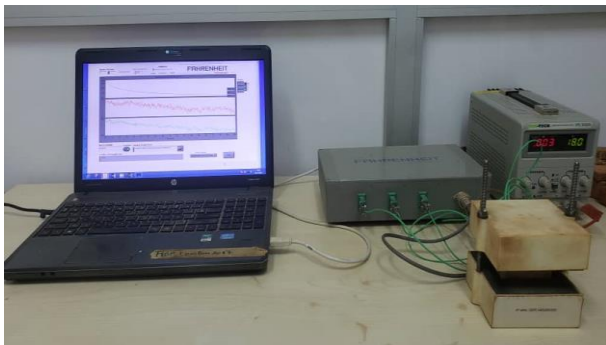
Fig.4. DesProTherm thermal characteristics measurement device.
