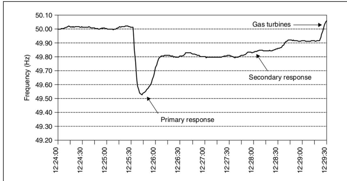
A 1,220 MW generation loss occurs in Great Britain, which has a total installed capacity of 65 GW;
