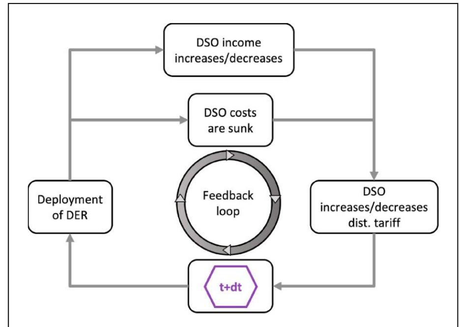
*Multi-agent interaction model with the feedback loop created by the deployment of residential PV panels and by the DSO's remuneration mechanism.<sup>1</sup>*
