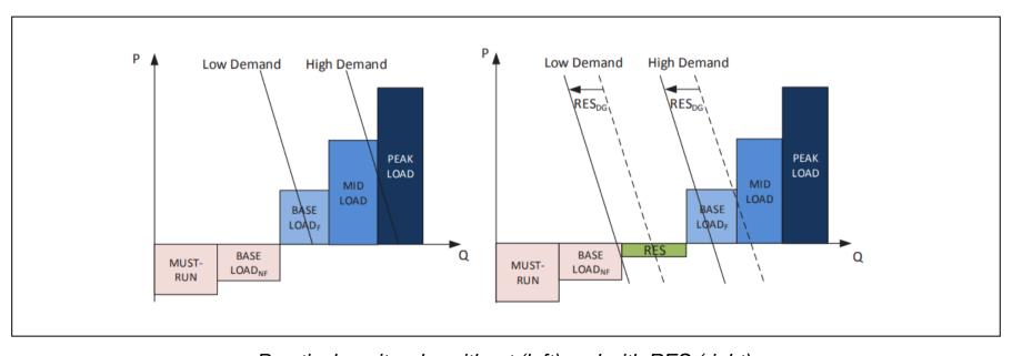
Practical merit order without (left) and with RES (right); RES<sub>( $\chi$ )</sub> expected renewable generation production of distributed nature; F flexible; NF non-flexible.<sup>1</sup>
