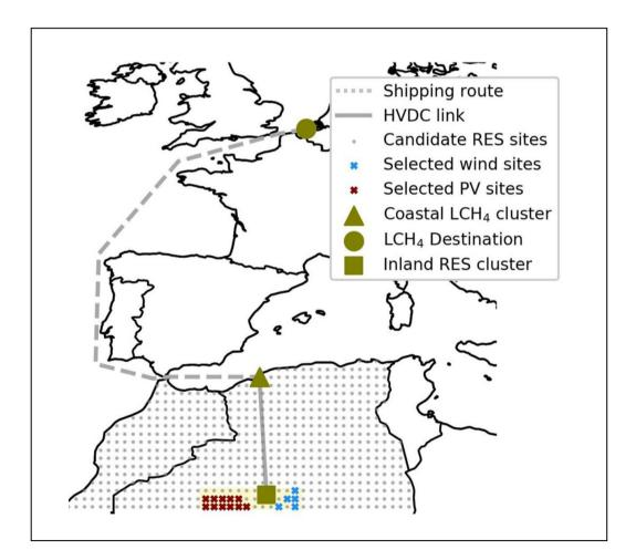
An example of an RREH is where solar and wind energy is collected in the Algerian desert, transmitted to the coast via an HVDC link, converted into carbon-neutral CH<sub>4</sub>, and then shipped to the EU.
