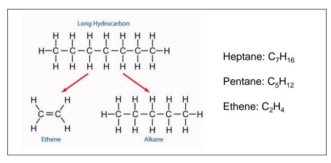
Example of catalytic cracking.1
