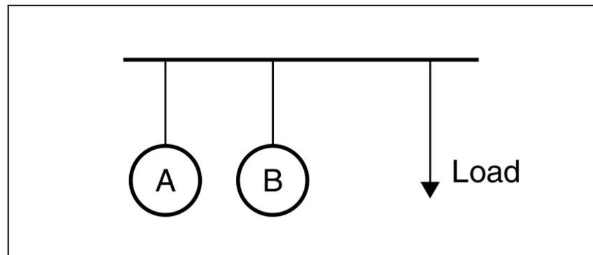
However, **the maximum load that can be handled securely is not 200 MW, but 100 MW!** This is because the operational limit is determined by the N-1 security criterion, which requires that the system must remain stable even if one generator fails.
