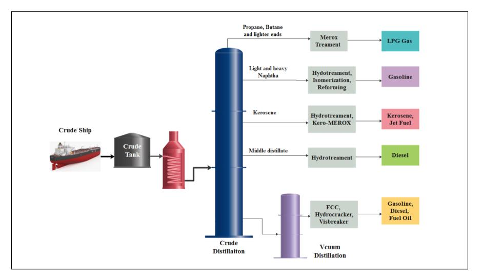
Hydrocarbon cracking is the process of breaking long hydrocarbon chains into shorter ones, yielding products that are easier to refine and use. The process requires high temperatures.
