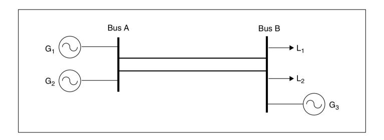
If the transmission lines between Bus A and Bus B can always transfer 500 MW, even under contingency conditions, this is acceptable.
