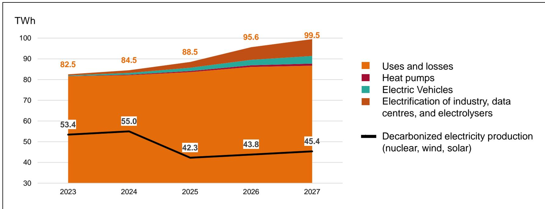
*Assumed future yearly electricity consumption in Belgium, by Elia (2023). There is a significant gap between decarbonized electricity production and the ever-increasing electricity consumption.<sup>1</sup>*
