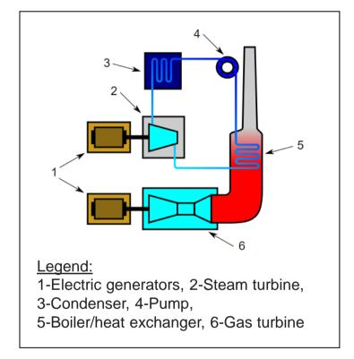
Working principle of a combined cycle power plant.<sup>1</sup>
