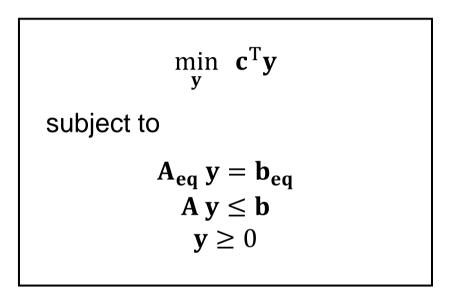
The compact form allows to easily encode the problem in a classical solver. Solving this problem, called the primal, provides the demand and generation schedules.
