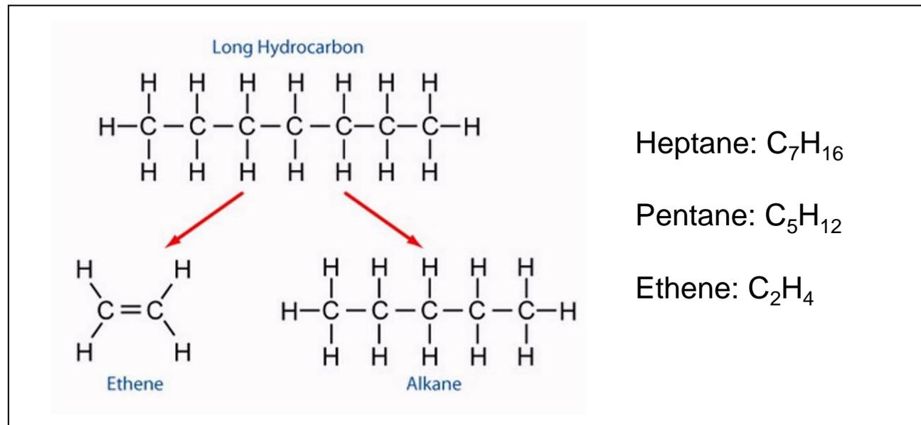
*Example of catalytic cracking.<sup>1</sup>*
