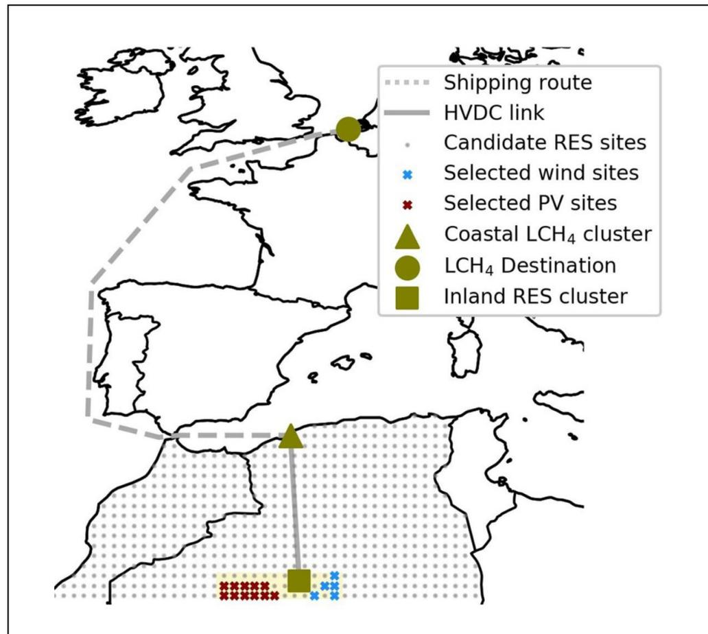
*An example of an RREH is where solar and wind energy is collected in the Algerian desert, transmitted to the coast via an HVDC link, converted into carbon-neutral  $CH_4$ , and then shipped to the EU.*
