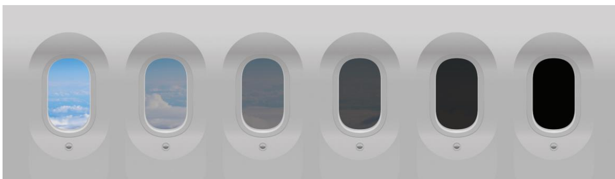
Figure 1.9: Progressive coloration of a Gentex electrochromic glazing used on an Boeing 787 Dreamliner window 32 .
