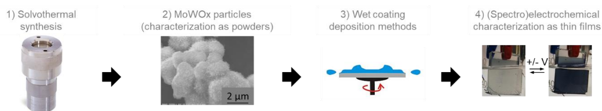
Figure 1.30: Schematic representation of the strategy used in the scope of this work, starting from solvothermally synthesized powders (1) 151 , which are characterized using various methods (2). Then, thin films are deposited using wet coating techniques (3) 152 , and finally, the obtained samples are characterized, in particular for their electrochromic performances (4).
