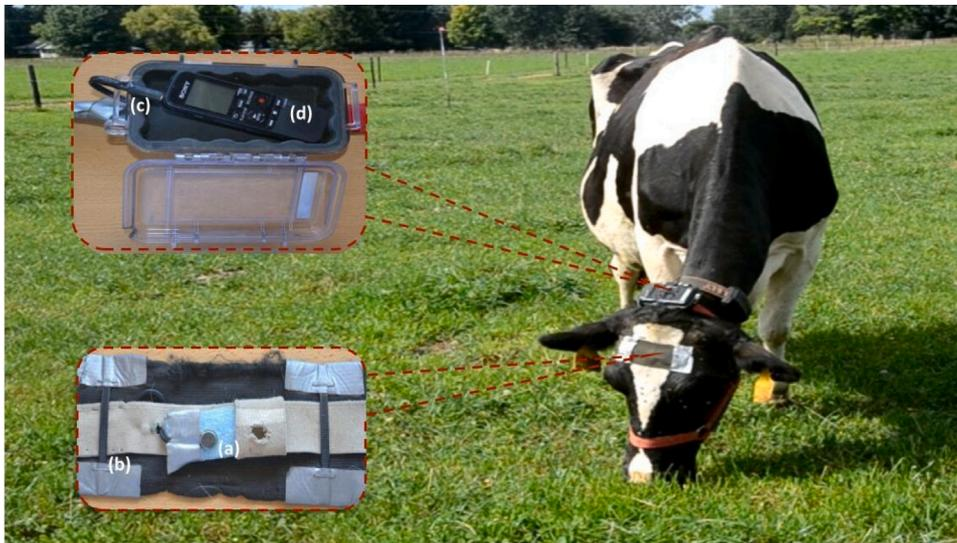
Fig. 3. Recording system used to record the acoustic signals composed of microphones (a) that are covered by rubber foam and an elastic headband (b), which are wired and plugged (c) to a digital recorder placed inside a waterproof case (d) attached to a neck halter.
