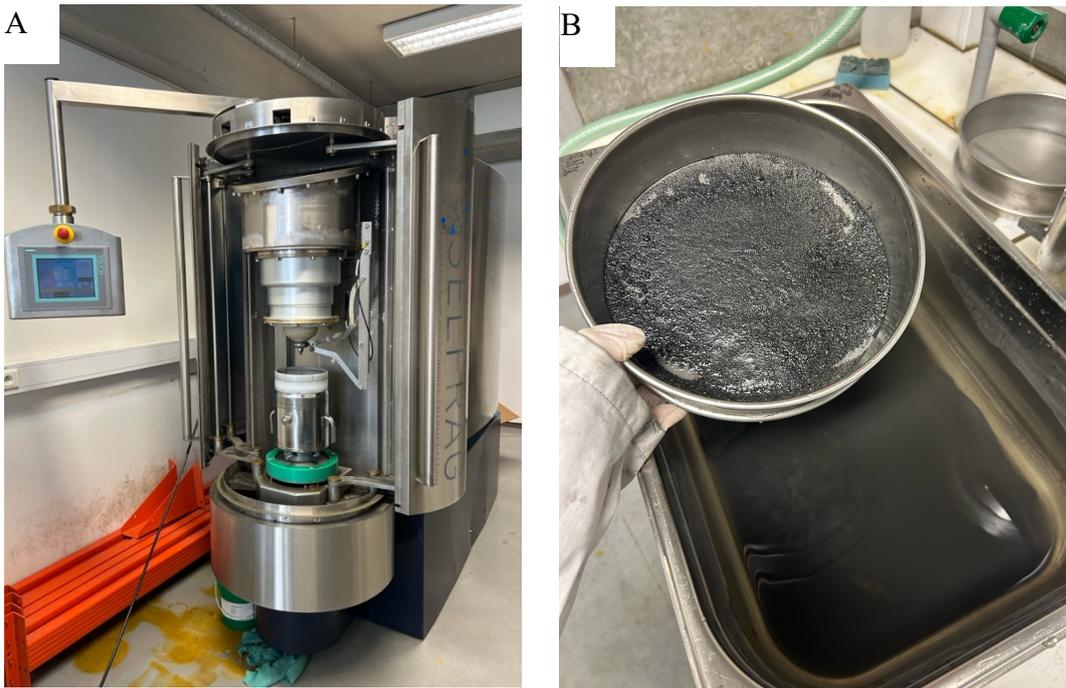
Annex 9. A. Selfrag apparatus. B. Sieve the Selfrag fragmented ore portion every 100 pulses approximately (150  $\mu\text{m}$ )
