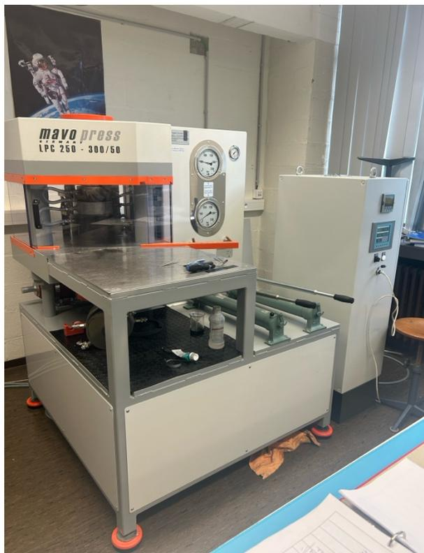
Annex 12. Piston cylinder apparatus, model MavoPress LPC 250-300/50 by Voggenreiter
