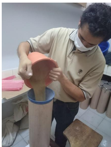
Figure A10.2 Preparation and setup of soil columns (a) and extraction of soil column sample after reclamation (b).
