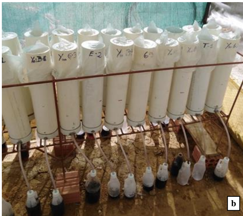
Figure 4.1 Soil column experiment to assess singly (a) and combined (b) organic and mineral amendments.
