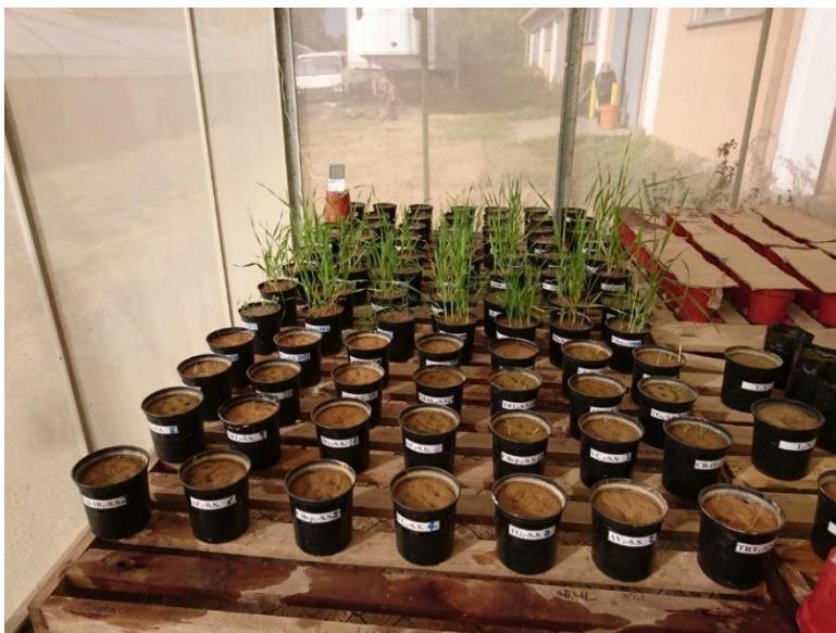
Figure A10.1 Pot experiment (by Castellón, D., 2018) to evaluate the effect of organic amendments in reclaiming a saline-sodic soil.
