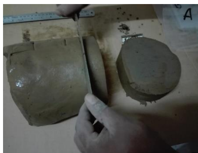
Figure A10.2 Preparation and setup of soil columns (a) and extraction of soil column sample after reclamation (b).
