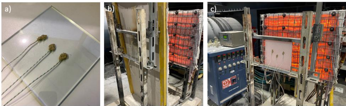
Figure 1 a) Sample with attached thermocouples, b) experimental setup with protecting plate before the start of the test, c) experimental setup with sample exposed to the heating.
