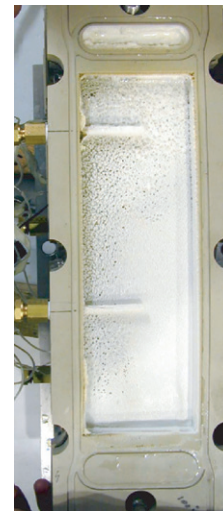
Fig. 6. Measurement of the temperature in the bulk during a 4-h fouling run: (a) evolution of the difference between the wall temperature and the bulk one and (b) photo of the thermocouples in the bulk after the run.
