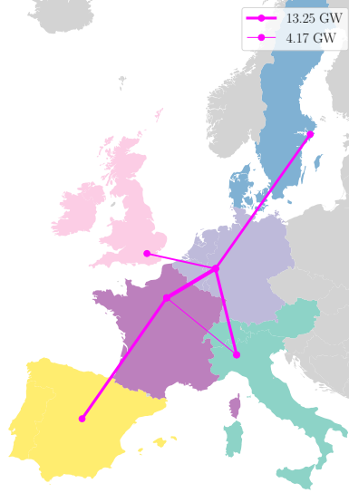
Figure 1: Aggregated regions considered in the model and network topology considered for hydrogen pipelines.
