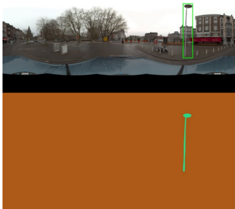
Figure 4. Resulting output from SAM based on the bounding box from the object detection
