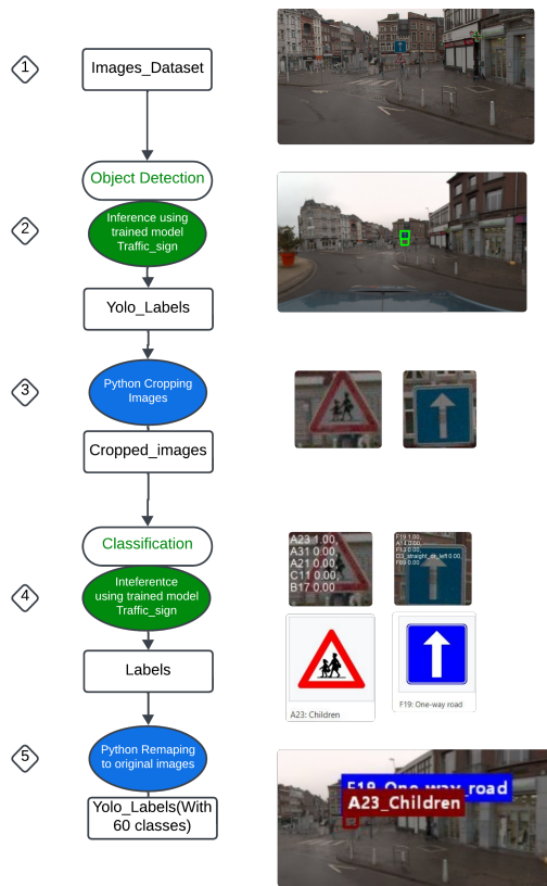
Figure 3. Cascaded Detection approach
