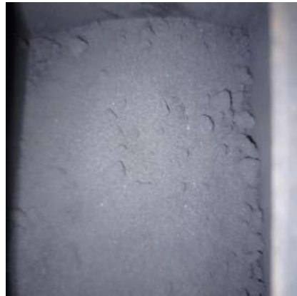
Substrate covered by carburizer
