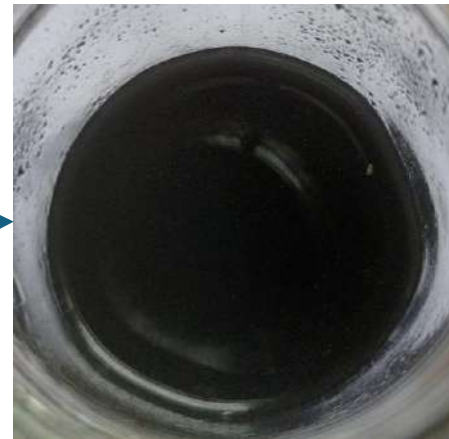
Bio-carburizer mixed with solution (2/1)
