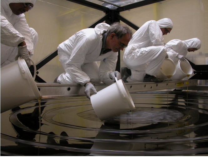
Fig. 2. Spincasting of the ILMT mirror. As the mirror rotates around its vertical axis, polyurethane is poured on the surface by members of the ILMT team (from left to right: Brajesh Kumar, Paul Hickson, François Finet and Arnaud Magette). After about half an hour, the resin has solidified.
