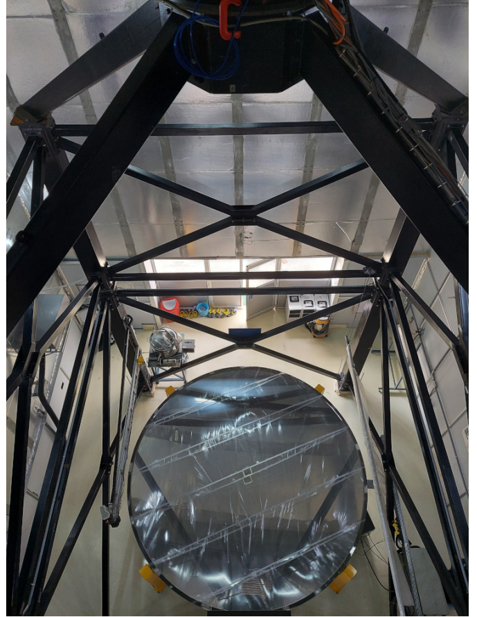
Fig. 3. Top view of the ILMT mirror surfaced with mercury and covered with thin assembled mylar films, which prevent the formation of ripples on the surface of the mercury. A tube is attached to the aluminium beam, just to the left of the edge of the mirror, to pump the mercury to and from the mirror and the tank visible at the top left side of the mirror. Near the middle left-hand side, one can see one end of a box containing charcoal to which a black tube is attached. It is used to evacuate the vapour when the mercury has just been transferred to the mirror (see text).
