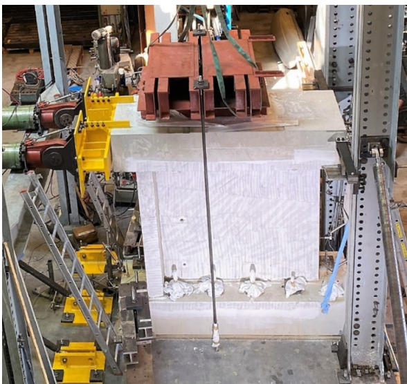
Fig. 4 Test setup of shear walls.
