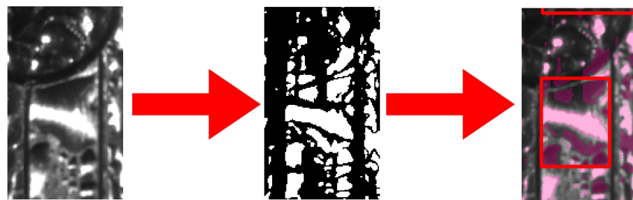
Figure 8. Sequence of Clustering the Drop Parts Starting From the Original Grooves Surface Image.
