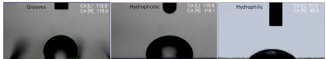
Figure 4. Contact angle (CA) measured on the top of the groove, as well as for the hydrophobic and hydrophilic.
