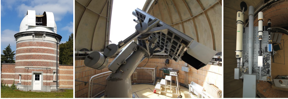
Fig. 2.1. USET station at the Royal Observatory of Belgium, located in Uccle, Brussels. Left picture: The dome. Middle picture: The equatorial table. Right picture: The 4 optical instruments (WL telescope, visual refractor, H\alpha telescope, Ca II K telescope (from the left to the right)).
