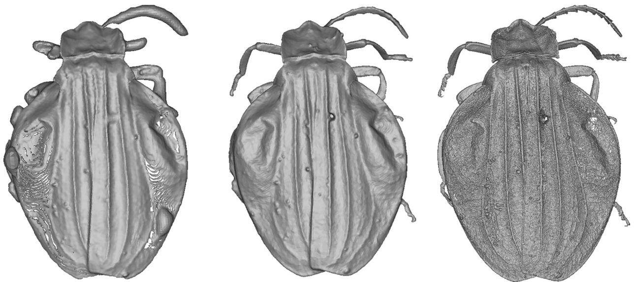
Fig 14. 3D model of Lycus rostratus . Left: SL. Center: SfM. Right: \mu CT.
