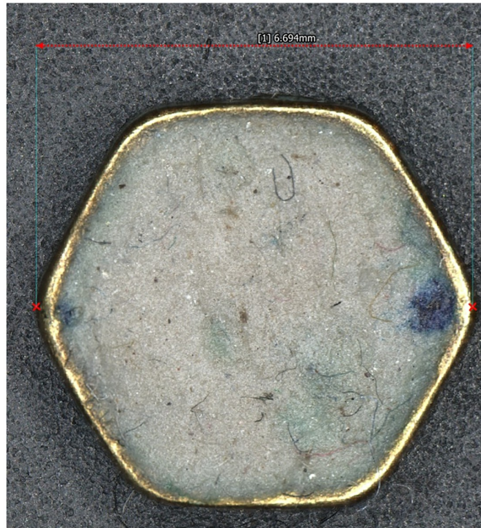
Fig 5. Hexagonal metallic bead used as a scale. The bead has been filled with plasticine to stay fixed on the needle.
