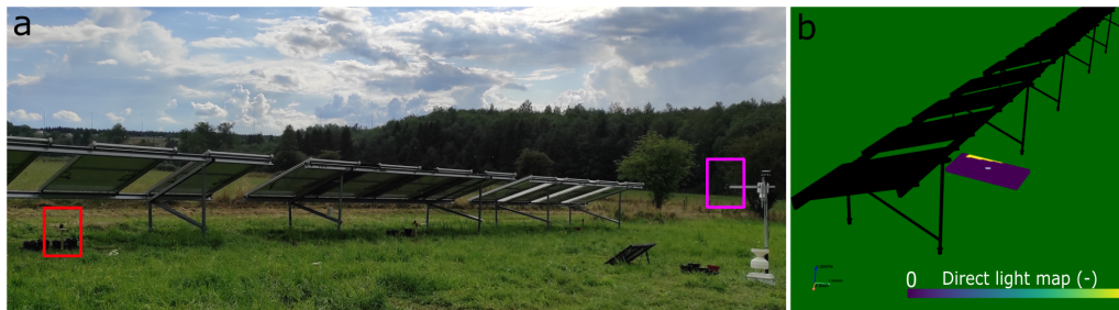
Fig. 4 (a) SigueSol agrivoltaic prototype and experimental set up with full sun condition pyranometer in purple and agrivoltaic pyranometer in red and (b) experimental set up reproduced in PASE
