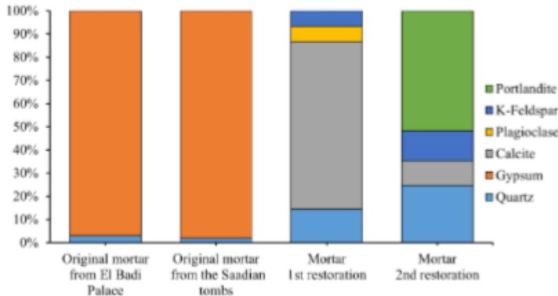
Mineralogical composition (XRD) of original mortars and those used in previous restoration phases.
