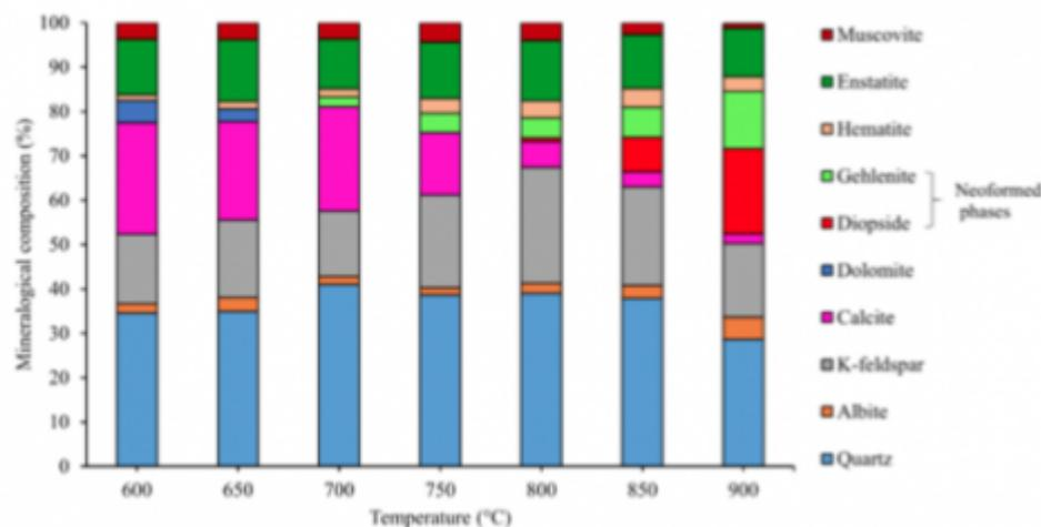
Mineralogical composition (XRD) of fired specimens
