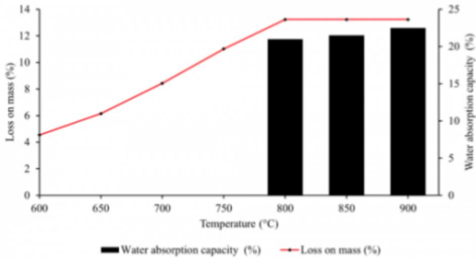
Evolution of loss on mass and water absorption capacity of the specimen in terms of firing temperature.
