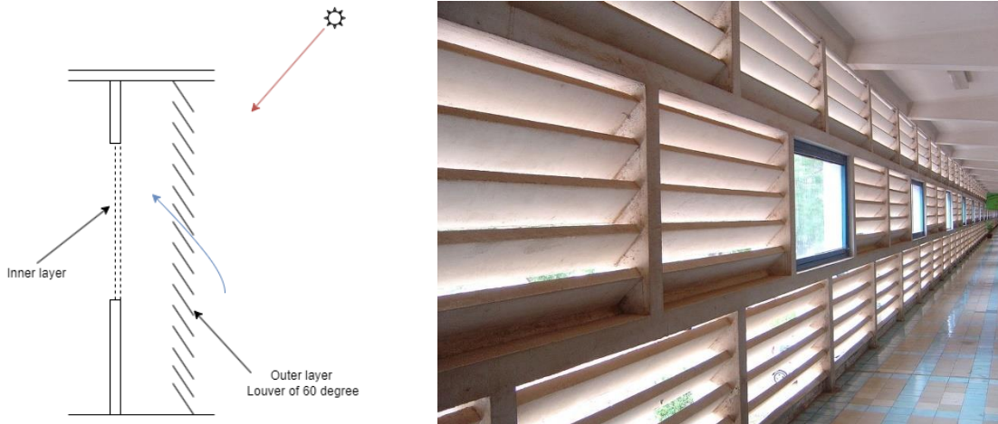
Figure 7-4: Example of using louver to create a double facade, source: Architectuul.
