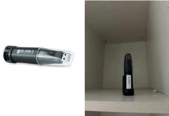
Figure 4-24: Data logger used to measure temperature and relative humidity.
