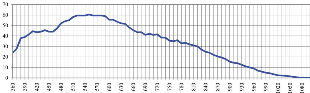
Figure 2. The quantum efficiency of OWL@OUKA CCD camera ProLine PL 16803. .
