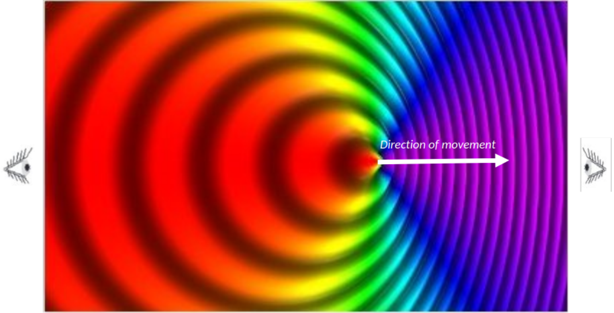
Figure 1.8: Hypothetical source of light moving to the right at a speed of 0.7c . The wavelengths are perceived shorter by the observer in the right and longer by the observer in the left the left. Credit: https://fr.wikipedia.org/wiki/Effet_Doppler_relativiste#/media/Fichier:Velocity0_70c.jpg
